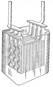
FIG. 9. Storage cell, in which energy is stored in chemical form through oxidation and reduction of lead electrically.
